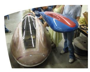
The nearly complete Infusion is on the ground, and the model is being held next to it. Minor instrumentation and a paint job are left on the to-do list.
